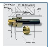
Compliance with the assembly instructions is extremely important for fulfilling the functions of the 2S cutting ring couplings. Improper handling leads to risks with regard to safety and freedom from leaks, which can also result in the complete failure of the coupling under certain conditions.
